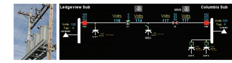
voltage that is adaptive to the dynamic changes that typical distribution circuits undergo. They also needed the ability to quantify the energy saved when the circuit is operating in the more precise lower or upper voltage band.
